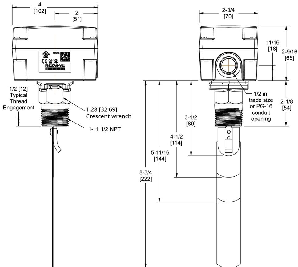
**Figure 3: Dimensions for F261 Low-Flow Switch, in. [mm]**
