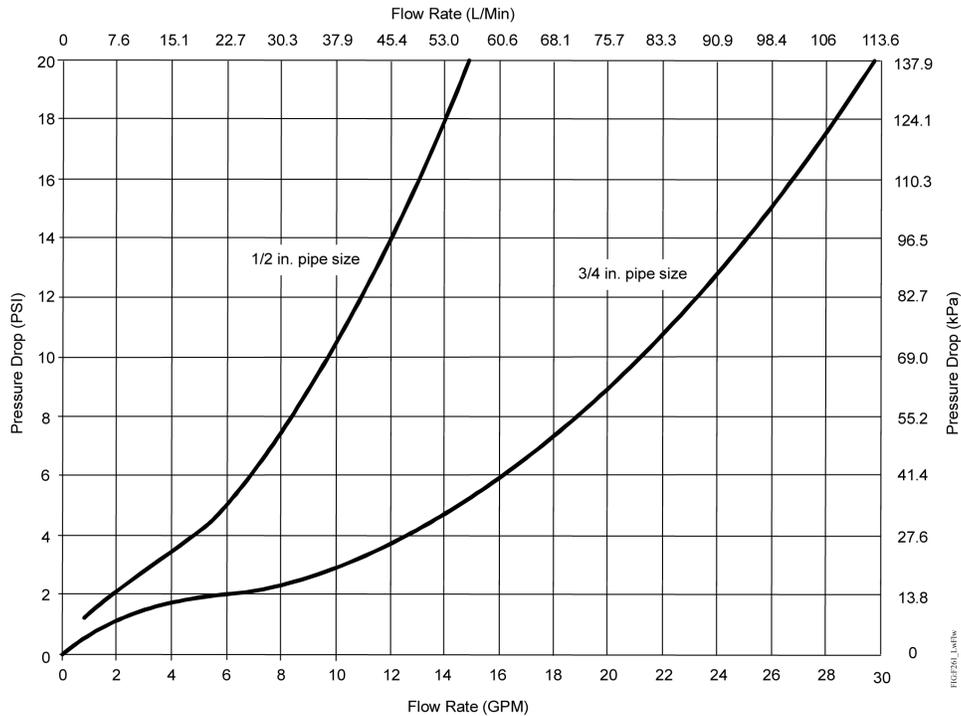
**Note:** This chart is correct for F261KEH-V01C, F261MEH-V01C, F261KFH-V01C, F261MFH-V01C low-flow switches.
