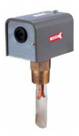
The F61KB-11C Liquid Flow Switches are single-Pole, Double-Throw (SPDT) flow switches that are used in liquid lines carrying water, ethylene glycol, or other liquids not classified as hazardous. They can be wired to energize one device and de-energize another device powered from the same source when liquid flow either exceeds or drops below the set flow rate.
