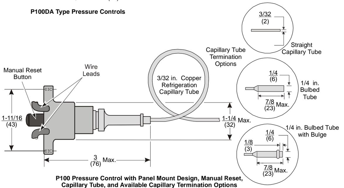
**P100 Pressure Control with Panel Mount Design, Manual Reset, Capillary Tube, and Available Capillary Termination Options**
