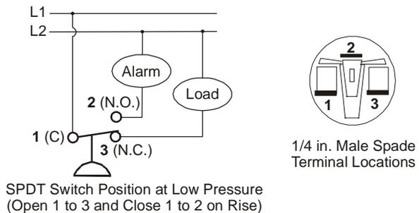
**Figure 4: Wiring Diagram and Terminal Locations for P100E Control Models with an SPDT Switch**
