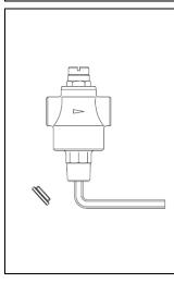
The final calibration of the pressure reducing valve must be performed with the hydraulic circuit completely full and with all the uses closed, otherwise false values would be obtained owing to the fact that the downstream pressure reduces in relation to the necessary flow rate, during any supply.
