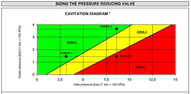
In order to avoid cavitation phenomena and therefore excessive component noise, we recommend choosing the number of pressure reducing valves necessary for a determinate pressure differential, according to the information in the "CAVITATION DIAGRAM". The cavitation diagram shows the three operating zones of the pressure reducing valve in function to the inlet and outlet pressures:
