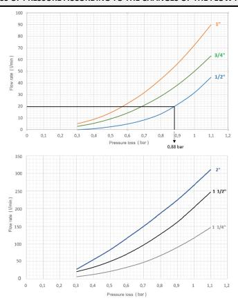
The graphic is prepared according to the conditions specified in EN 1567 standard. (Input pressure 8 bar - Output pressure 3 bar)
