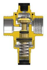
The water pressure reducer is designed to reduce the pressure of high pressure mains water to prevent damage to the installation and to the devices connected to the installation.
